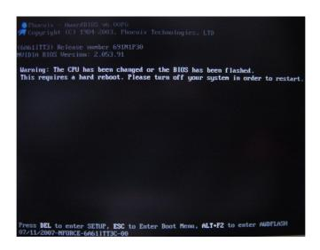
(3) Press [DEL] key to enter BIOS setup when system is boot up. Use the arrows to highlight the item "LOAD OPTIMAL SETTINGS" then press "Enter". System will ask "Load Optimal Settings (Y/N)?" Press "Y" and "Enter" keys to confirm.
