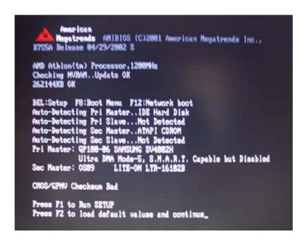
(3) Press [F1] key to enter BIOS setup when system is boot up. Use the arrows to highlight the item "LOAD OPTIMAL SETTINGS" then press "Enter". System will ask "Load Optimal Settings (Y/N)?" Press "Y" and "Enter" keys to confirm.
